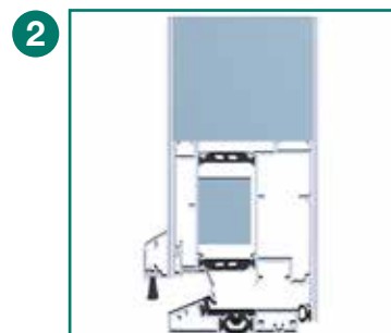
Threshold with heat barrier and three sealing points
