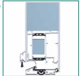
Threshold with heat barrier and three sealing points
